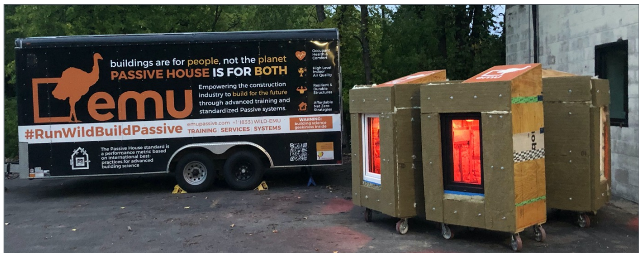
Image 33: Resiliency Test carried out at the end of one of Emu's Passive Design/Build Boot Camps.
